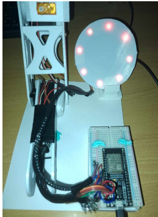
Fig. 12. Warning light was illuminated when emergency.
