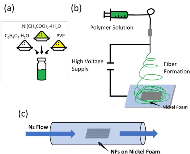
**Fig. 1.** Schematics of (a) the polymeric solution, (b) electrospinning set-up, and (c) annealing process in a tube furnace.
