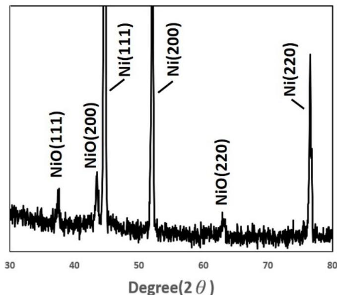
**Fig. 3.** XRD pattern of binder-free porous NiO-NF fibers.
