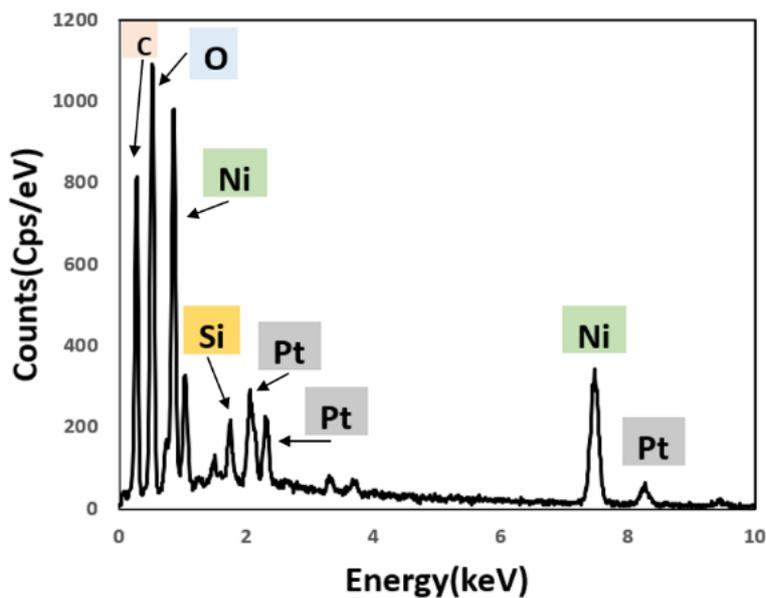
Fig. 4. EDX spectrum of binder-free porous NiO-NF fibers.
