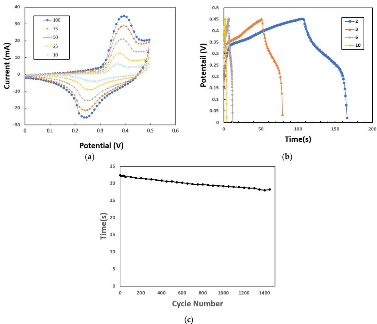
Fig. 5. (a) Cyclic voltammety, (b) galvanostatic charge/discharge, and (c) cycling performance of fabricated Ni-NFs.
