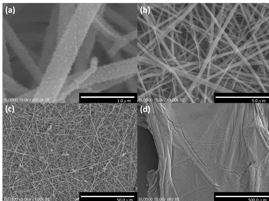
**Fig. 2.** Morphology of electrospun porous Ni-NFs on Ni foam was observed through SEM magnified by (a) 50,000, (b) 90,000, (c) 100,000, and (d) 600,000.
